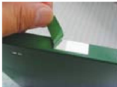
After the paint is dry, the maskin tape is removed, exposing the conductive Al surface.
