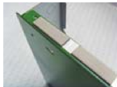
Conductive cushion gasket is applied on the exposed Al surface.
