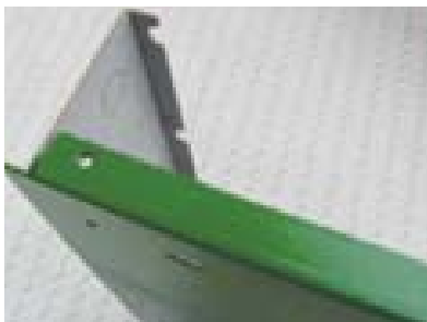
Conductive maskin tape is applied to the case edge and painted over.
